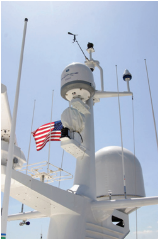
Figure 4 — KVH 60cm Antenna allows mounting on high masts above superstructure, which reduces blockages
